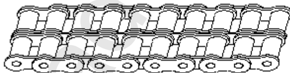
Standard roller chain, two-strand (also available with three and four strands)
